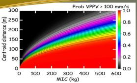
Probabilistic analysis: Plot shows the probability of exceeding 100 mm/s on infrastructure for a given charge weight and distance.
